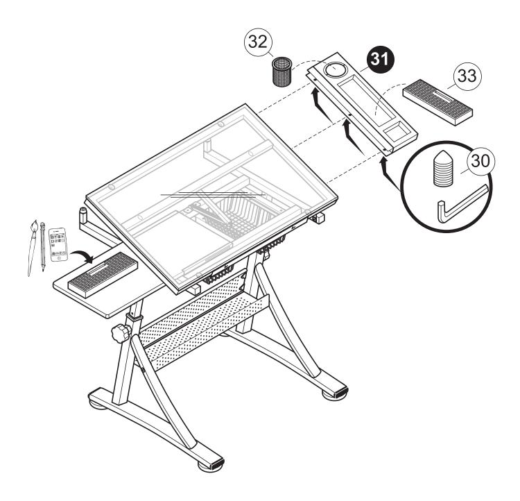
Slide Metal Tray (31) over edge of table (frame and glass), and secure using Allen Screws (30) **(do not overtighten)**. Insert Cup (32) and Foam Organizer Tray (33) into slots. Foam Tray can also be placed on shelf as a mobile organizer.
